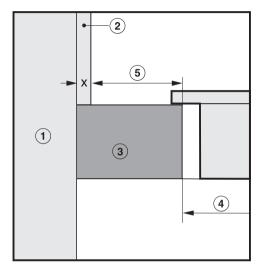
If the niche cladding is made from a **non-combustible material** (e. g. metal, natural stone, ceramic tiles) a minimum safety distance (5) of 50 mm less the thickness of the cladding must be maintained between the cut-out and the cladding.
